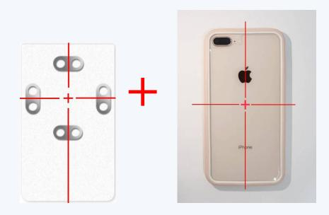
Applying sequence (1): From top to bottom, set the adhesive docking sheet at the center of the device.
